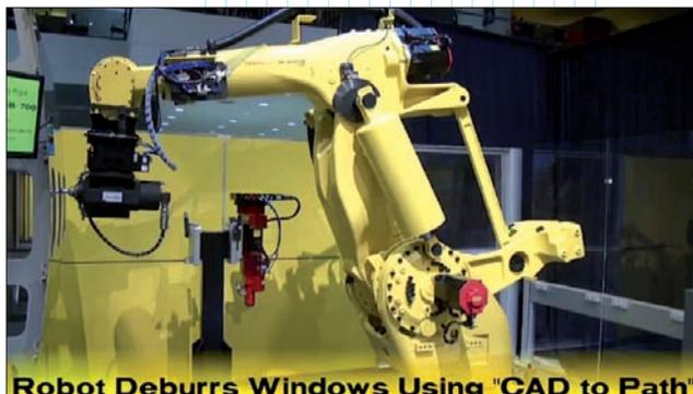
**Robot Deburrs Windows Using “CAD to Path”**
